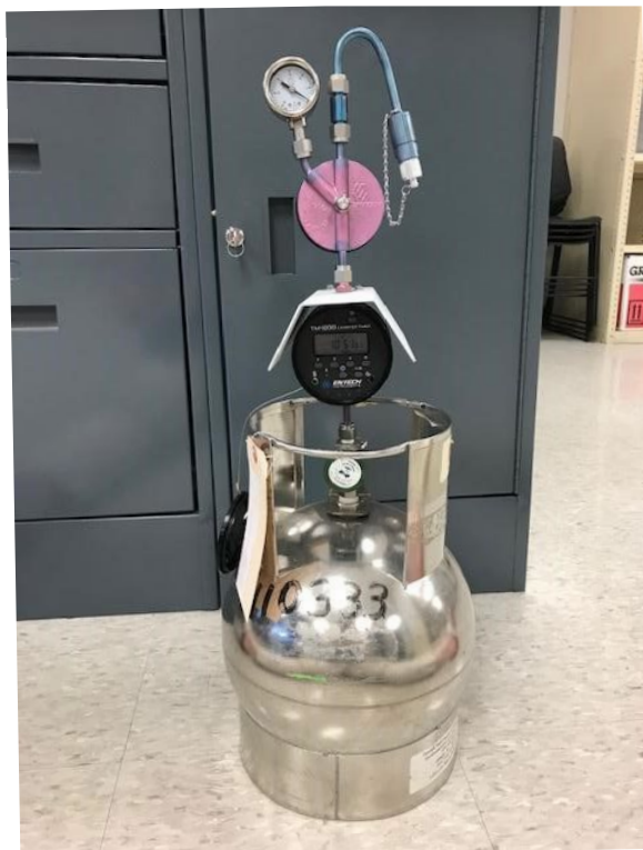
Figure 11.2-1 Entech CS1200E Passive VOCs Sampler Set-Up
