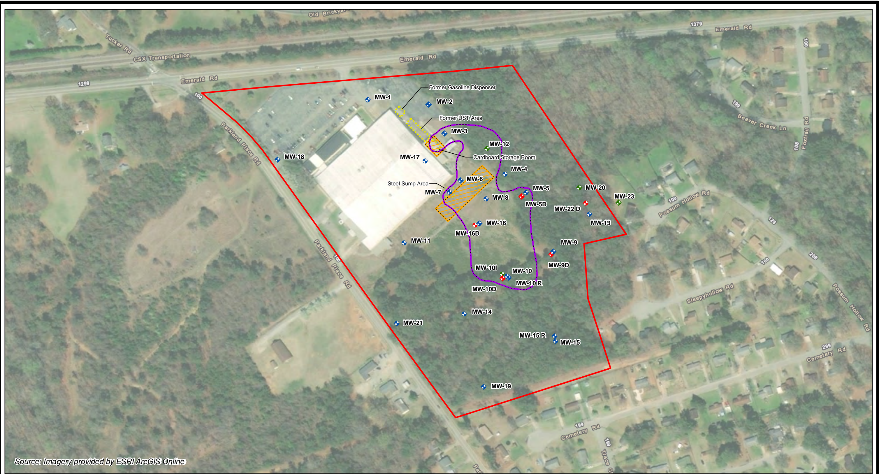
Figure 17 Alternative 6 - Excavation and Disposal Combined with In Situ Chemical Oxidation (ISCO) Using PersulfOx ® with MNA/ICs
