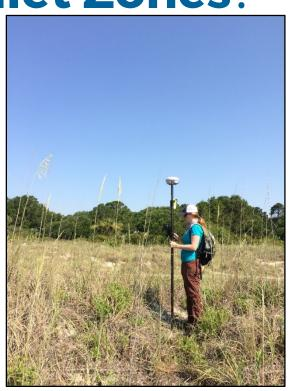
Field data were collected by agency experts using a Trimble R6 RTK GPS unit and the South Carolina Real Time Network.
