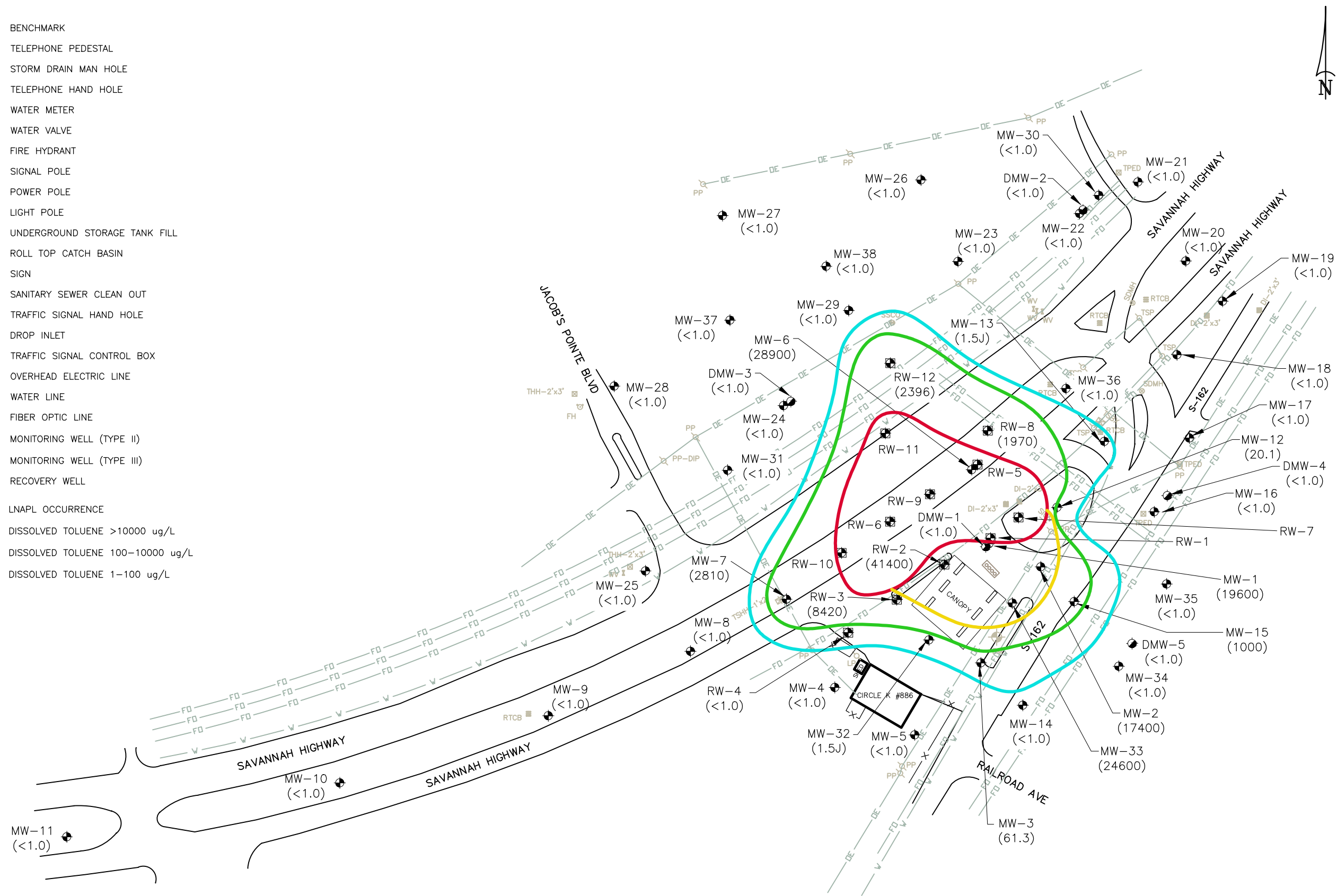
FIGURE 6 TOLUENE ISOPLETH MAP FOR GROUNDWATER - OCTOBER 2021 CIRCLE K #2720886 4315 SAVANNAH HIGHWAY RAVENEL, SOUTH CAROLINA
