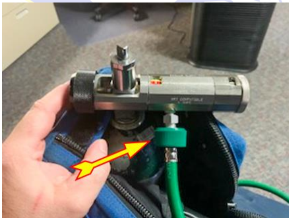
Figure 4. Connection of the Oxygen Tube From Nitrous Oxide Regulator to Oxygen Cylinder
