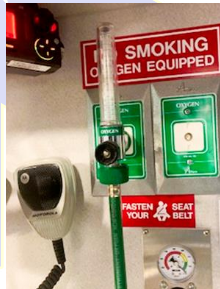
Figure 6. Preparation of the Ambulance Oxygen Supply. Attach Oxygen Line from NitroNox Regulator to Standard Oxygen Connector
