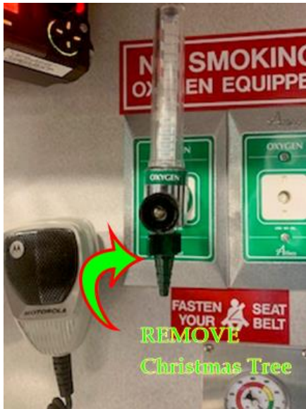
Figure 5. Preparation of the Ambulance Oxygen Supply. Remove attached Christmas Tree.
