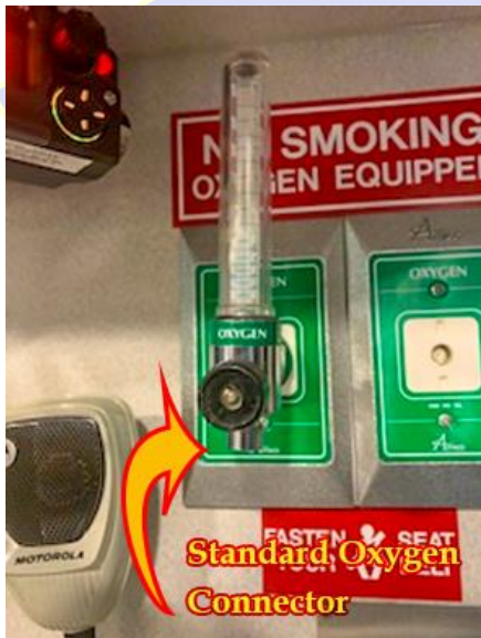
Figure 6. Preparation of the Ambulance Oxygen Supply. Attach Oxygen Line from NitroNox Regulator to Standard Oxygen Connector
