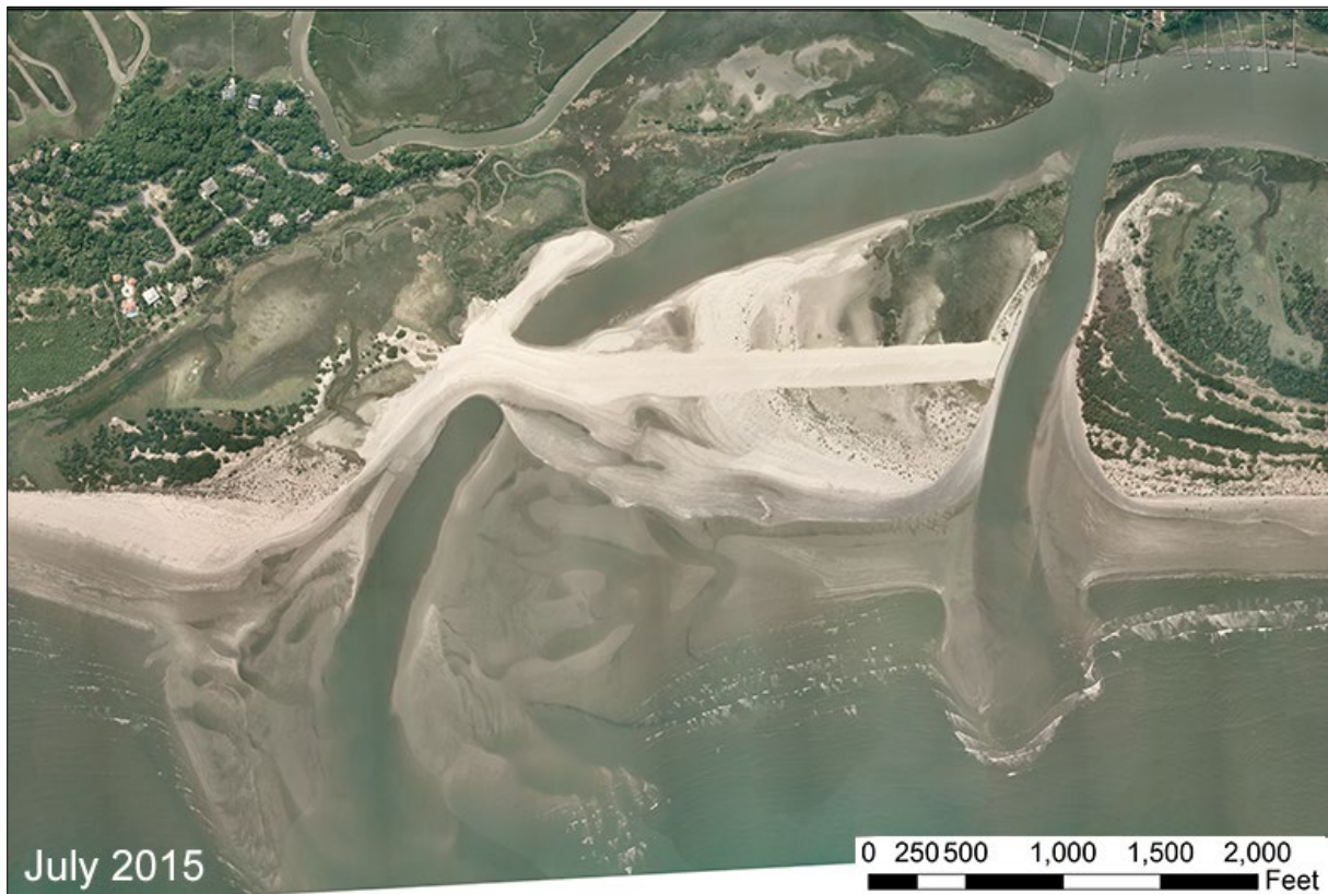
FIGURE T-12. Captain Sams Inlet after inlet relocation in June 2015. Kiawah spit is to the right and Captain Sams Creek is at the upper right corner of the image. The orthorectified aerial photo was prepared by Independent Mapping Consultants Inc (Charlotte NC).
