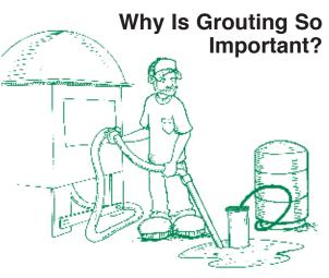
Properly installed grout is one of the most important protective features of your well. It ensures that contaminants from the surface do not seep down into the water you will drink. Grout is made of cement or bentonite.
