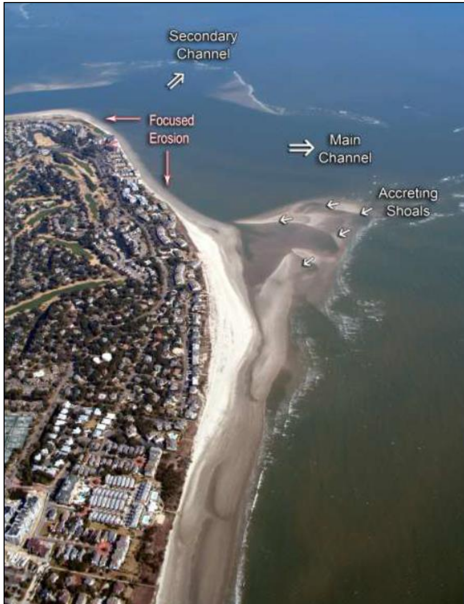
Figure 3. February 2007 view northeast toward Dewees Inlet (CSE, 2015a). Migrating inlet shoal leads to a wide beach immediately landward of the migrating shoal, and focused erosion adjacent to the location of shoal attachment.
