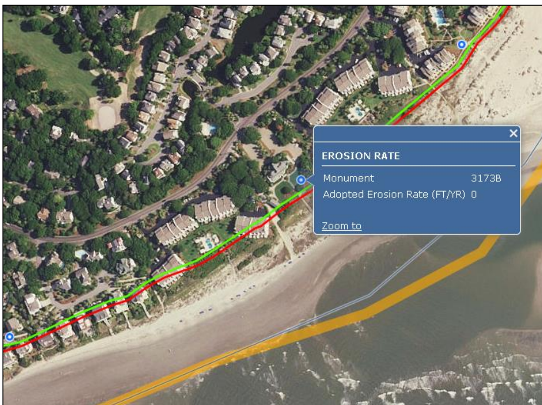
Figure 19. Example of long-term accretion and 20ft minimum setback distance, with DHEC OCRM Baseline and Setback Line landward of existing development.
