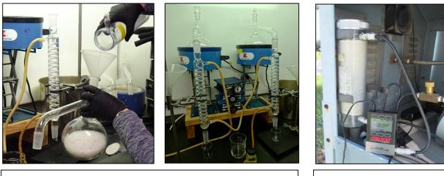
Collecting atmospheric moisture from silica gel through distillation
