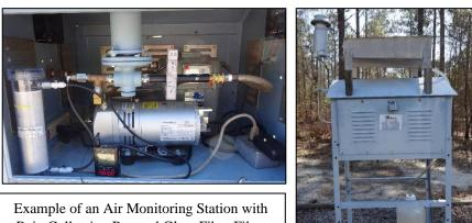
Rain Collection Pan and Glass Fiber Filter (on top) and Silica Gel Column (inside)
