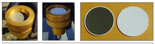
Glass fiber filter being collected for total suspended particulates: Used filter (left) vs. unused filter (right)
