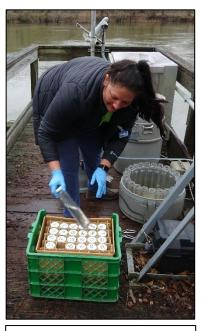
Collecting samples to be tested for tritium using the early detection system at SV-118
