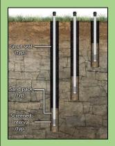
**NETWORK WELLS** are single wells at a specific location screened in a specific aquifer.
