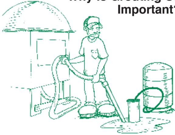
Properly installed grout is one of the most important protective features of your well. It ensures that contaminants from the surface do not seep down into the water you will drink. Grout is made of cement or bentonite.
