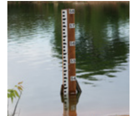
Figure 23. Lake level gauge
