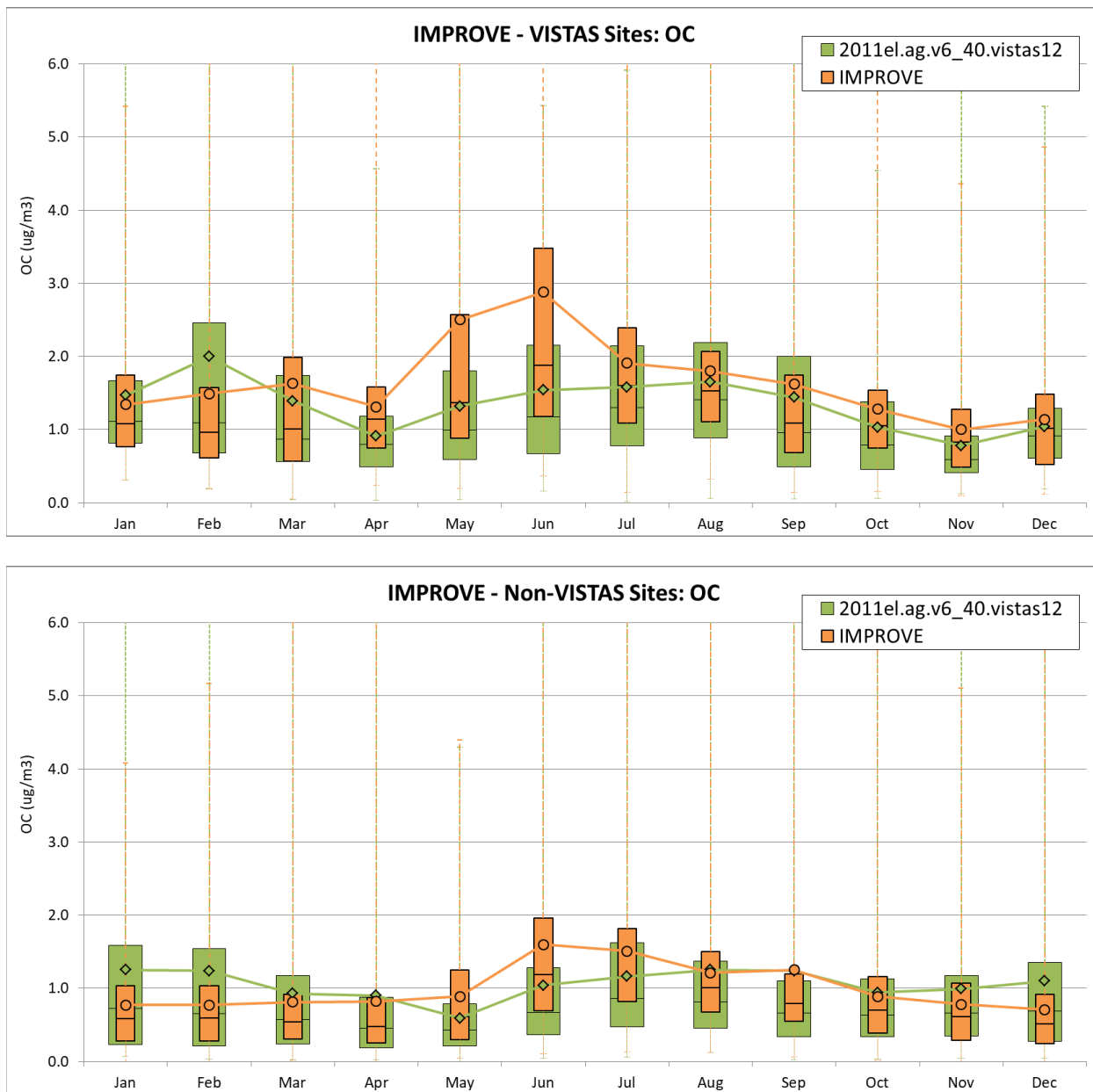
Figure 7-23. Boxplot Comparisons of Model Predictions and IMPROVE Organic Carbon (OC) Observations for Each Climate Region by Month.
