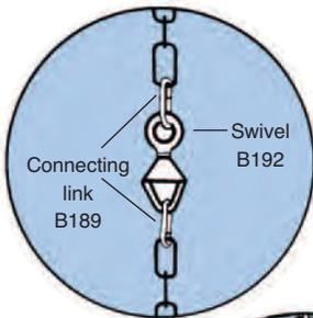
**Use swivels to cut chain wear and increase buoy performance.** Wind, wave, and current action causes buoys to rotate. This rotation, if severe, can cause chain or cable to twist, which will eventually submerge the buoy, increase chain wear, and increase the load on the anchor.
