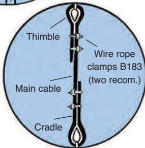
**Correct cable clamp assembly.** Note from the sketch that the cradle is tightened against main cable. This is the correct assembly method to insure against the clamps, slipping while in service. Be sure to tighten nuts down, alternating from side to side frequently. Thimbles should be assembled so they are firmly trapped within the cable loop.
