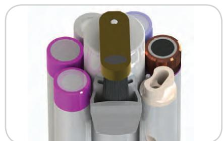
Wiper keeps sensors clear of biofouling
