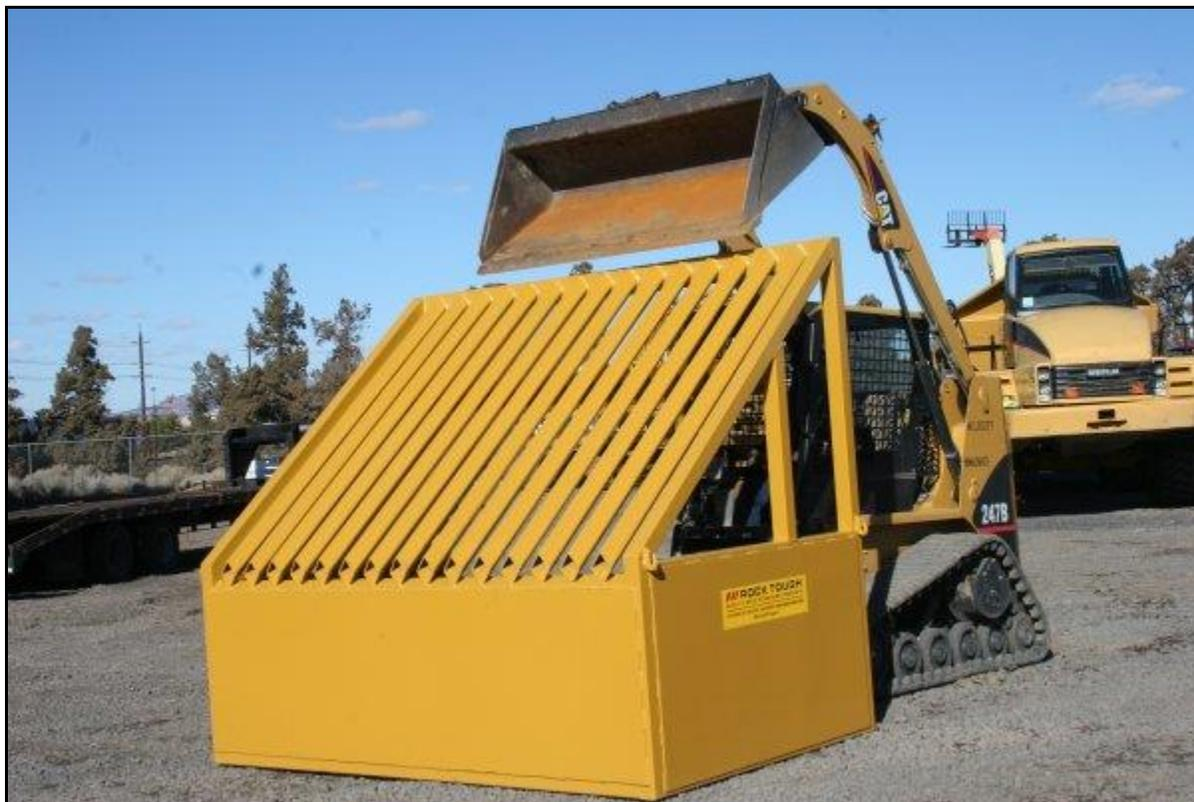
Figure 6. Example of a bar sorter
