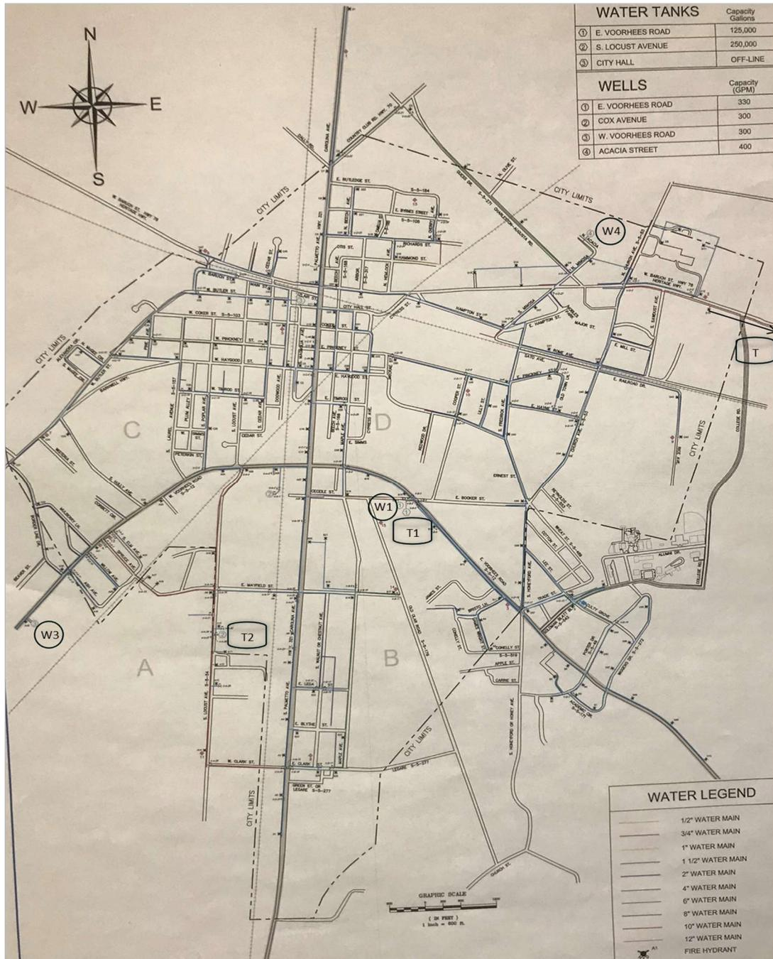
FIGURE 2. Denmark water system schematic.
