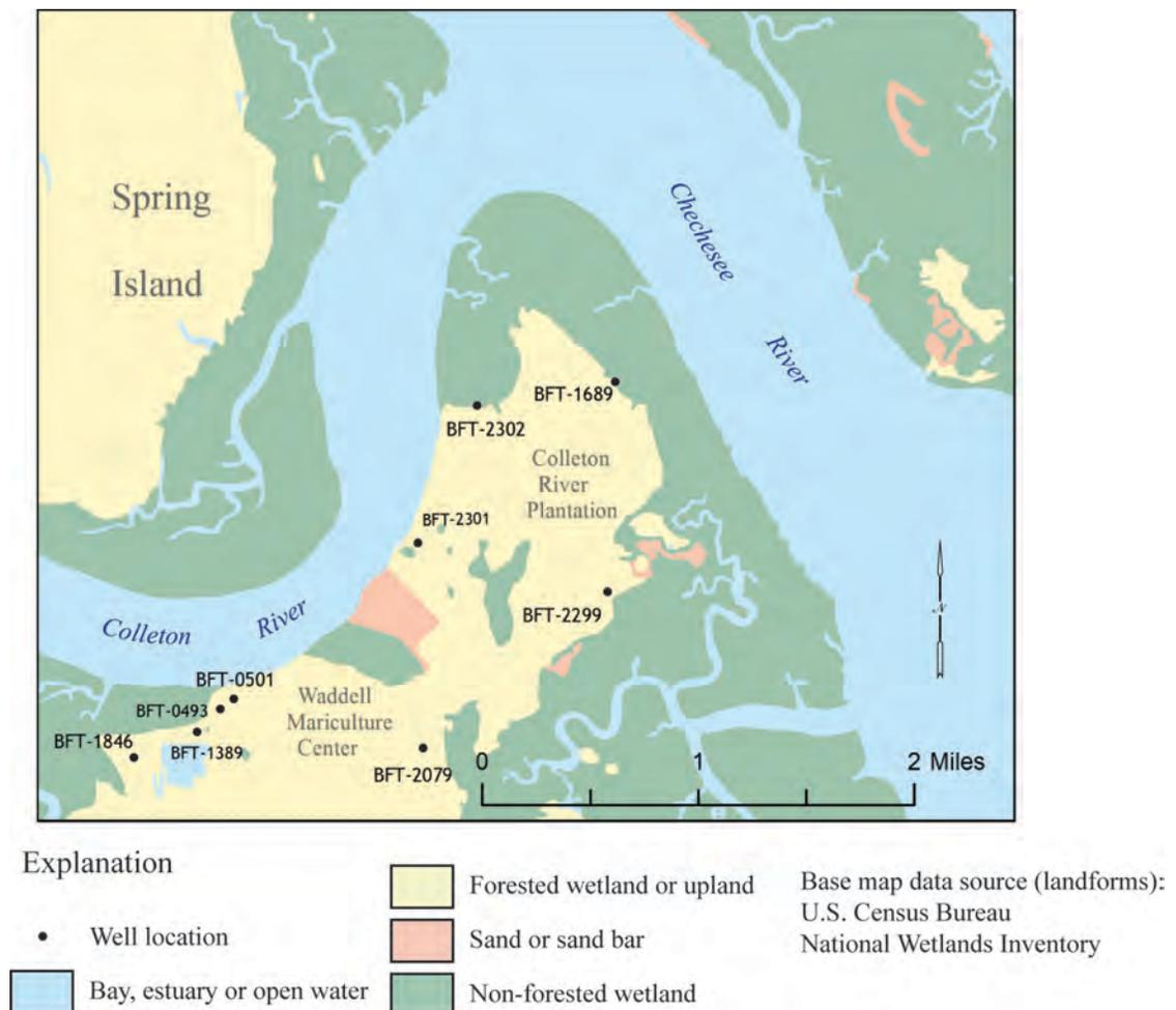
Figure 46. Locations of Upper Floridan aquifer test wells in the Colleton River Plantation area, S.C.
