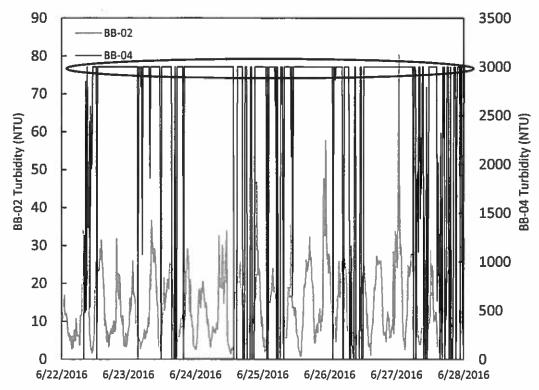
Continuous monitoring Turbidity data from within the same field area. The record from Station BB-04 site is the result of turbidity sensor failure during deployment and is typical of obviously erroneous data. Please note the extreme difference in Turbidity scales between the primary and secondary vertical axes as well as the flat shape of the BB-04 profile across the top highlighted by the red circle.
