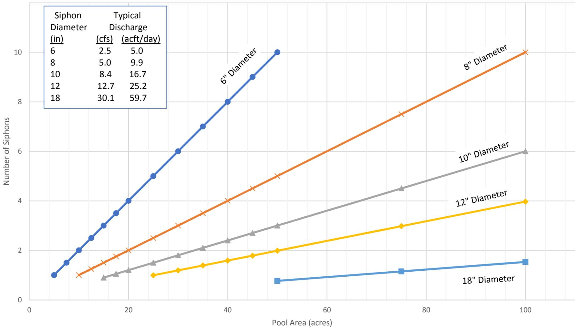
\*Chart represents typical conditions described in DSG 101 document, Use of Siphon Quantity Chart. Performance may vary based on driving head, siphon parts, or change in pond area as water is drawn down.
